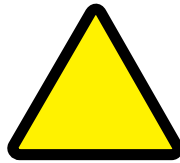
2.1 CAUTION Potential Hazard (black on yellow)
